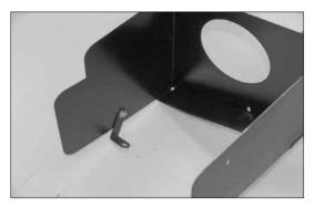
12. Install the "L" bracket (070632) onto the heat shield as shown with the provided hardware.
