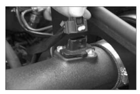
29. Reconnect the mass air sensor electrical connection.
