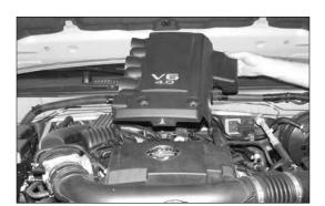
4. Lift firmly on the engine cover to dislodge it from the mounting grommets, and then remove the cover from the engine as shown.
