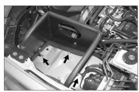
19. Install the heat shield assembly into the vehicle and secure with the provided hardware to the air box mounting locations.
