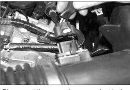
2. Disconnect the mass air sensor electrical connection and unhook the harness from the air box.
