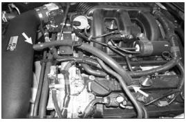
24. Attach the provided crank case vent hose to the valve cover and K&N<sup>®</sup> intake tube as shown and secure with the provided hose clamps.
